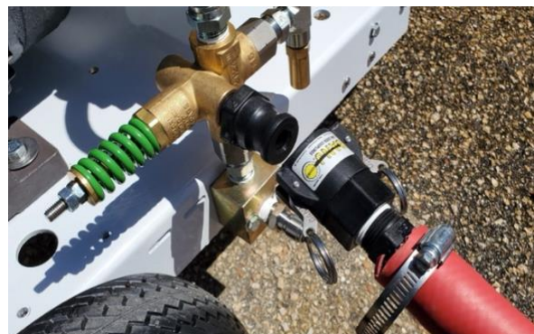
Figure # 6 – By-Pass Hose connection
