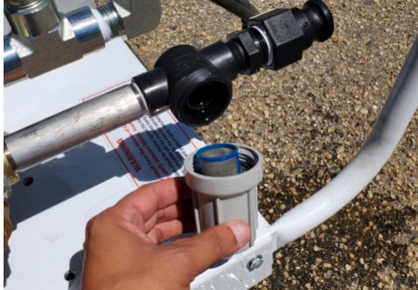
Figure # 1 – Inlet Water Strainer
