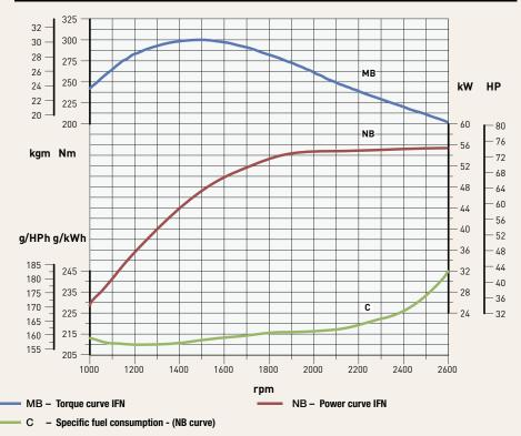
Power ratings refer to engines equipped with air filter, standard muffler, after running-in period at ambient conditions of  $+25^{\circ}$ C, relative humidity 30% and 1 bar. Derating depending on applications.
