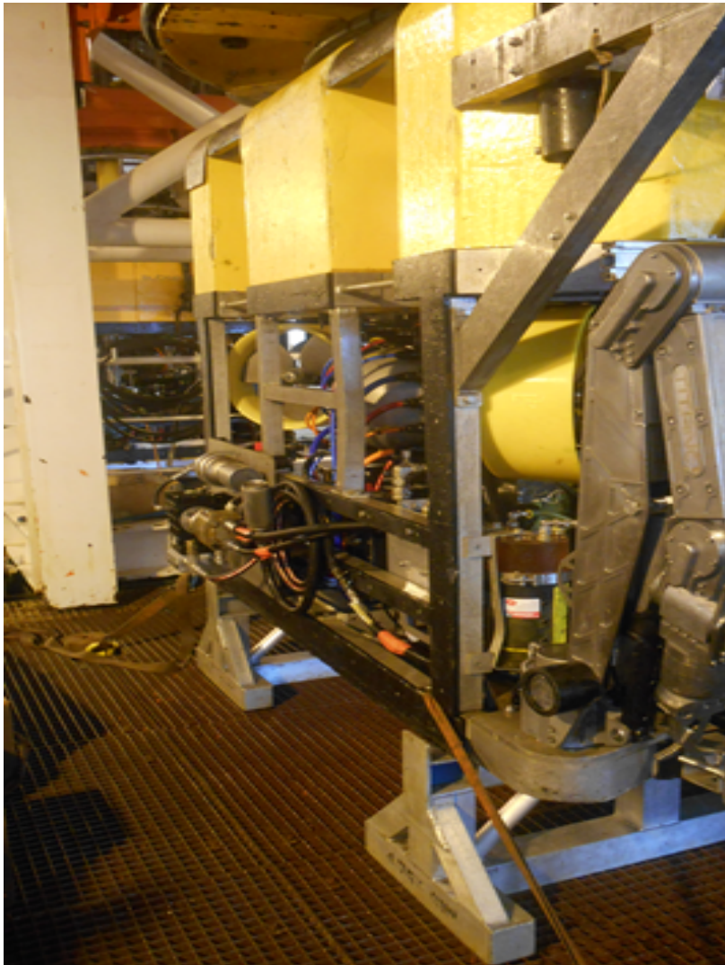
Picture 2. Showing the cavitation jetter fitted to the outboard starboard side of H27.
